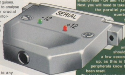
This illustration shows what the 'dongle' should look like when finished. Note the LEDs protruding through the plastic casing
